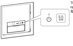
The operating mode switches each time the emergency operation button is pressed.
