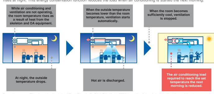
The out door temperture (OA) setting can be selected either 17°C or 28°C by using Dip-Switch (SW2-7) in the LOSSNAY control box. Refer to the Instillation Manual for more information. \*Do not use the night purge function if fog and heavy rain is expected. The entry of rain water may occur in the night.
