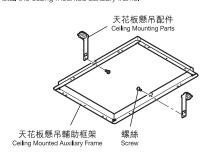
4 將浴室換氣暖風機主體伸進天花板懸吊輔助框架。 Place the Bathroom Thermo-Ventilator into the ceiling mounted auxiliary frame.
